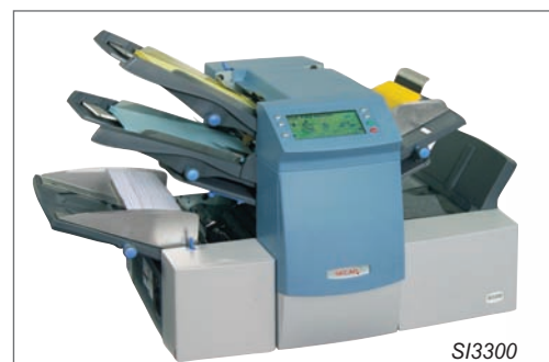
The SI3300 and SI3500 process routine office, promotional and transactional mail. The SI3300 operates at speeds up to 3,000 pieces per hour. It offers a standard envelope feeder holding up to 100 envelopes. The SI3500 processes up to 3,500 pieces per hour and has a robust envelope feeder which holds up to 325 envelopes.
