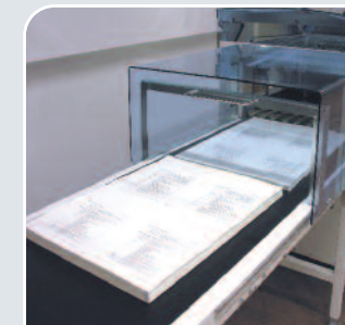
Long sheet stacker LS6-28" can handle 3.5" up to 28" sheets
