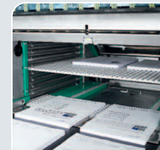
Non-stop LS6 stacker eliminates printer stops
