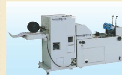
The best-selling SPF-11/FC-11 bookletmaker has become established as an industry standard. The SPF-11 is equipped with two Magnatec stitching heads (maximum 4 heads). This unit is best suited for short to medium run lengths.
