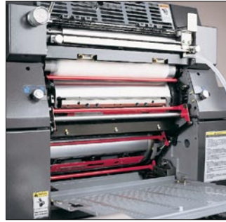
Straight-edge plate clamps with positioning pins are featured. Cylinder safety bars and covers protect fingers.
