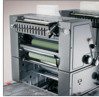
Segmented Lever Actuated Ink Fountains add a great deal of automation for increased productivity and fewer wasted sheets.
