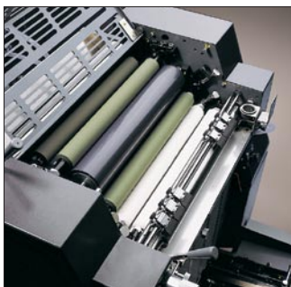
Each printing head has 16 inking rollers including 3 form rollers of differing diameters. The 'stepless' inking and 5-roller molleton dampening system allows maximum control of the printed image.
