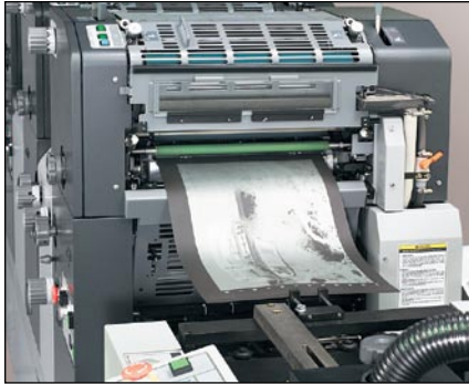
Semi-automatic plate loading increases accuracy thereby reducing the amount of registration adjustments.
