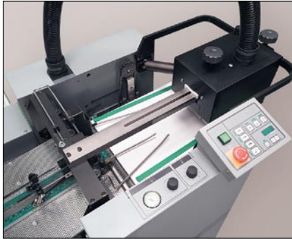
The stream feeder on the 4995A-ICS provides smooth, dependable feeding of papers ranging from onionskin to heavy card stock.
