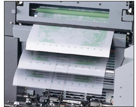
Professional features such as semi-automatic plate changing and the computerized Ink Control System (ICS) help efficiently manage the increasing amount of multi-color work.
