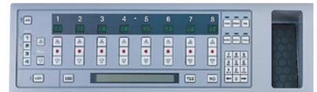
Professional features such as semi-automatic plate changing and the computerized Ink Control System (ICS) help efficiently manage the increasing amount of multi-color work.
